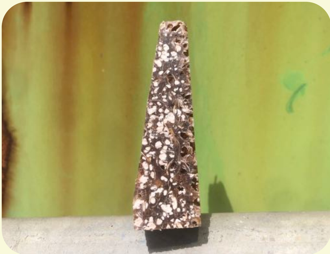
Wedges made from dissolved polystyrene and extraction.
