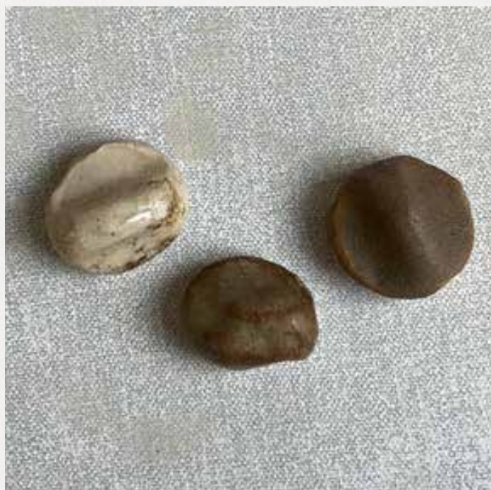
Fig. 43, ashe glaze test tiles, chrome oxide, nickel oxide and rutile dark.
