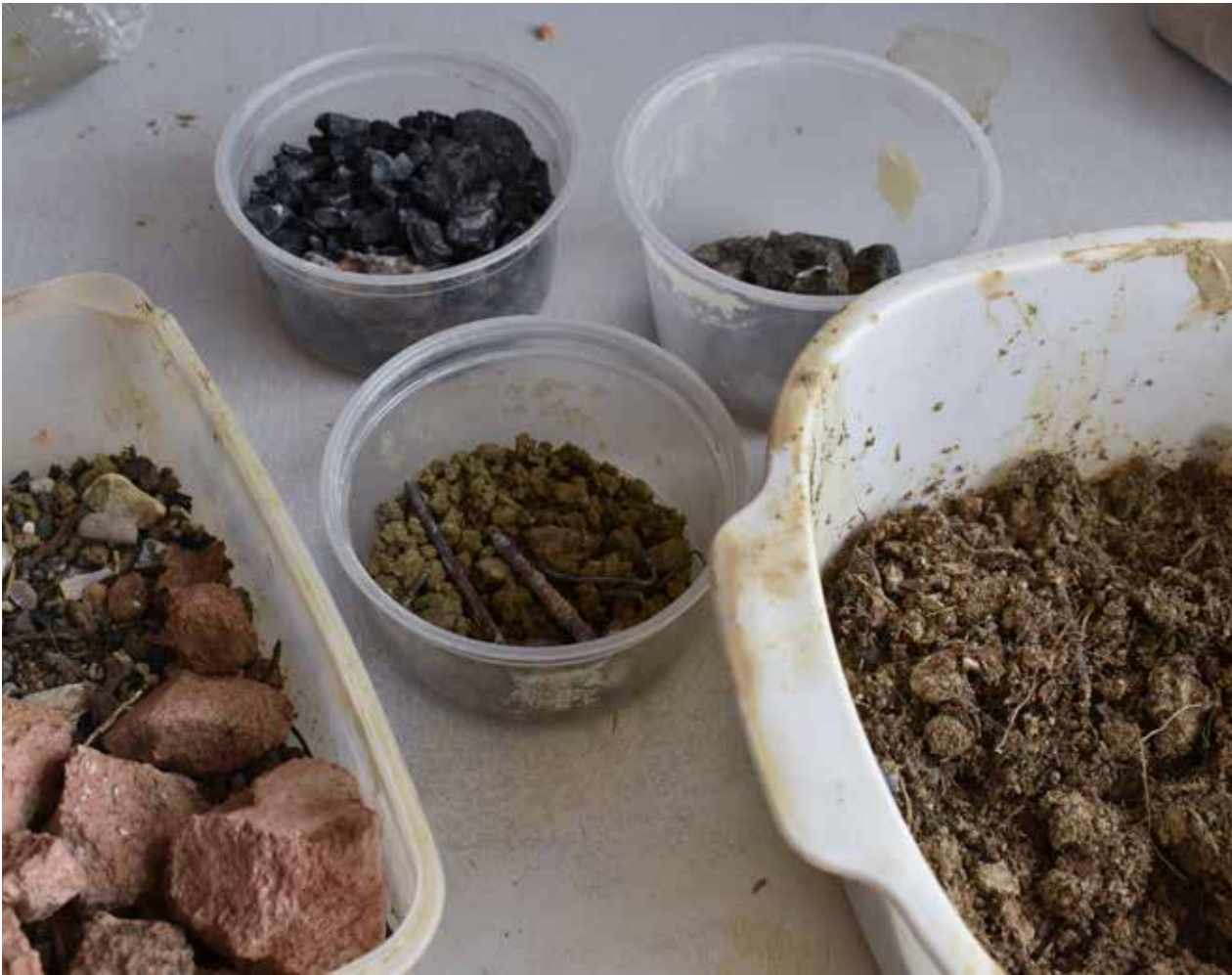
Debris, found when processing the clay. From left to right: Soil, rocks, red brick, twigs, nails, dry unprocessed Portslade Clay.
