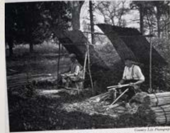
70. Cleaving and pointing with the billhook.
