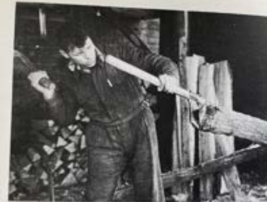
91. Driving the tree with a mallet to cleave triangular segments for girth bars.
