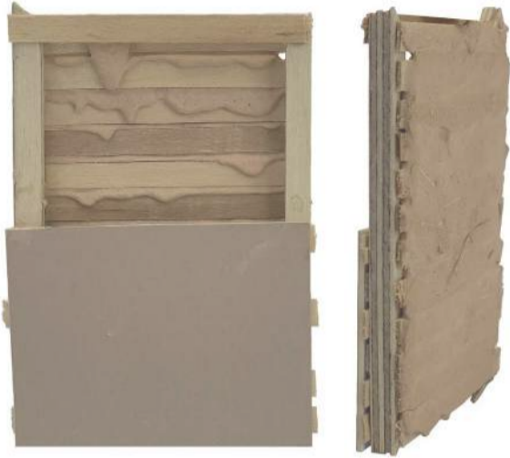
Experimentation of Site's Lathes and Plaster
