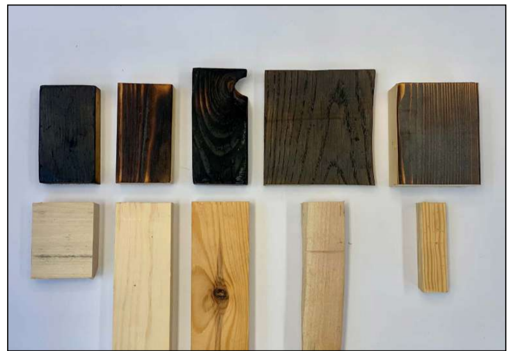
Testing / Charring Wood Types
