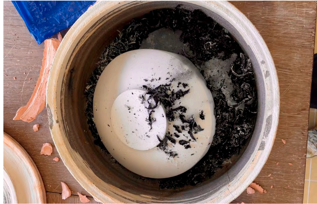
LEFT: SAGGAR FIRED SLIPCAST FORMS, CERAMICS WORKSHOP ABOVE: SAGGAR POT WITH SYCAMORE SHAVINGS, CERAMICS WORKSHOP
