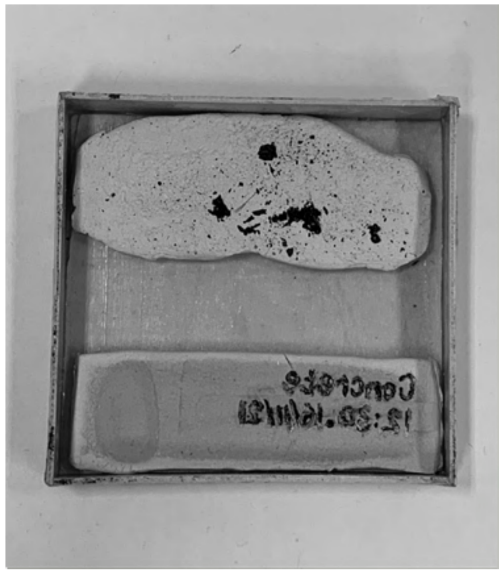
'In the Mould' Thumb Print and Time Stamp. Time stamp is mirrored so that when it is Plaster Casted, the text would be the correct way round.
