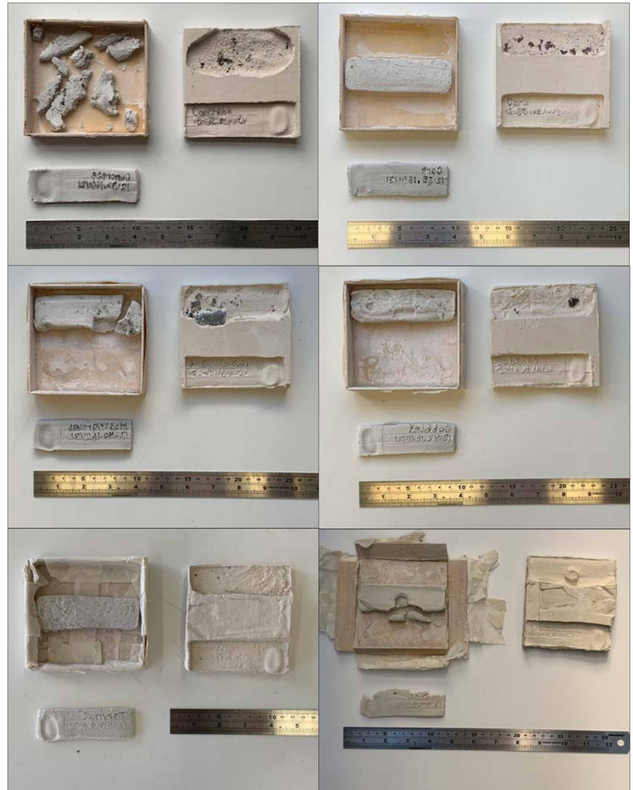
'Outcomes' The Plaster Casting leaves accurate markings and traces of site materials, transferred from the clay imprints. Embossed Time Stamp and Thumb Print
