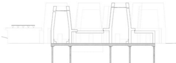
CONCRETE PILES WITH CONCRETE BASE
