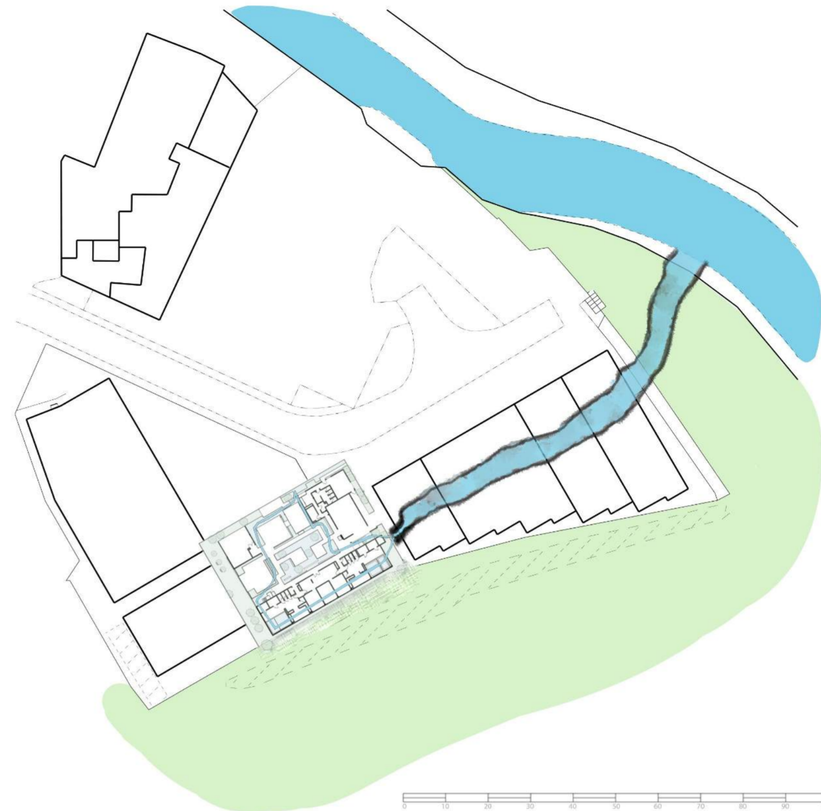
Drawing of Naman Retreat Spa on site exploring water supply from the river
