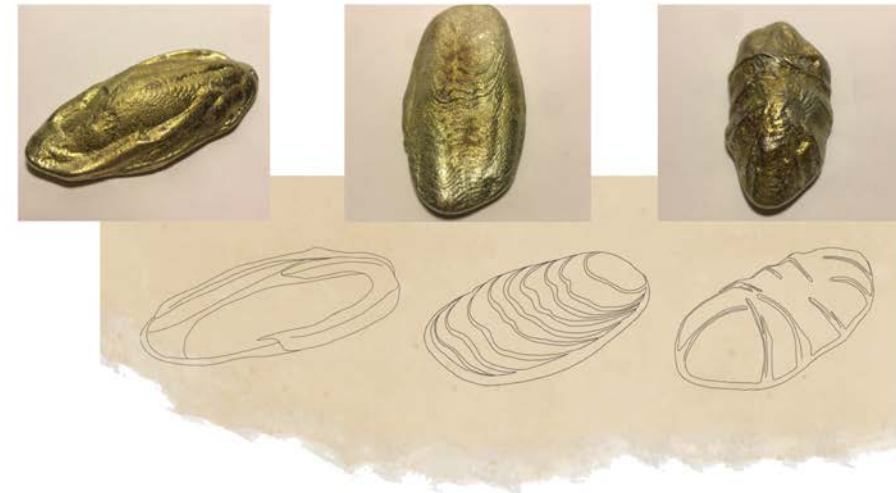
Cuttlefish castings made with pewter.
