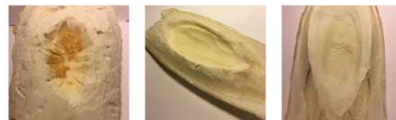
Cuttlefish bones carved out to create a mould for pewter.
