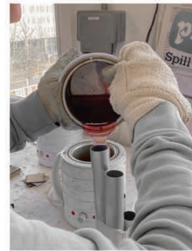
2. Pouring glass wax in the metal tubes used as molds.
