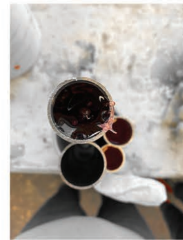
3. Letting the glass wax cool down and take a cylindrical form.
