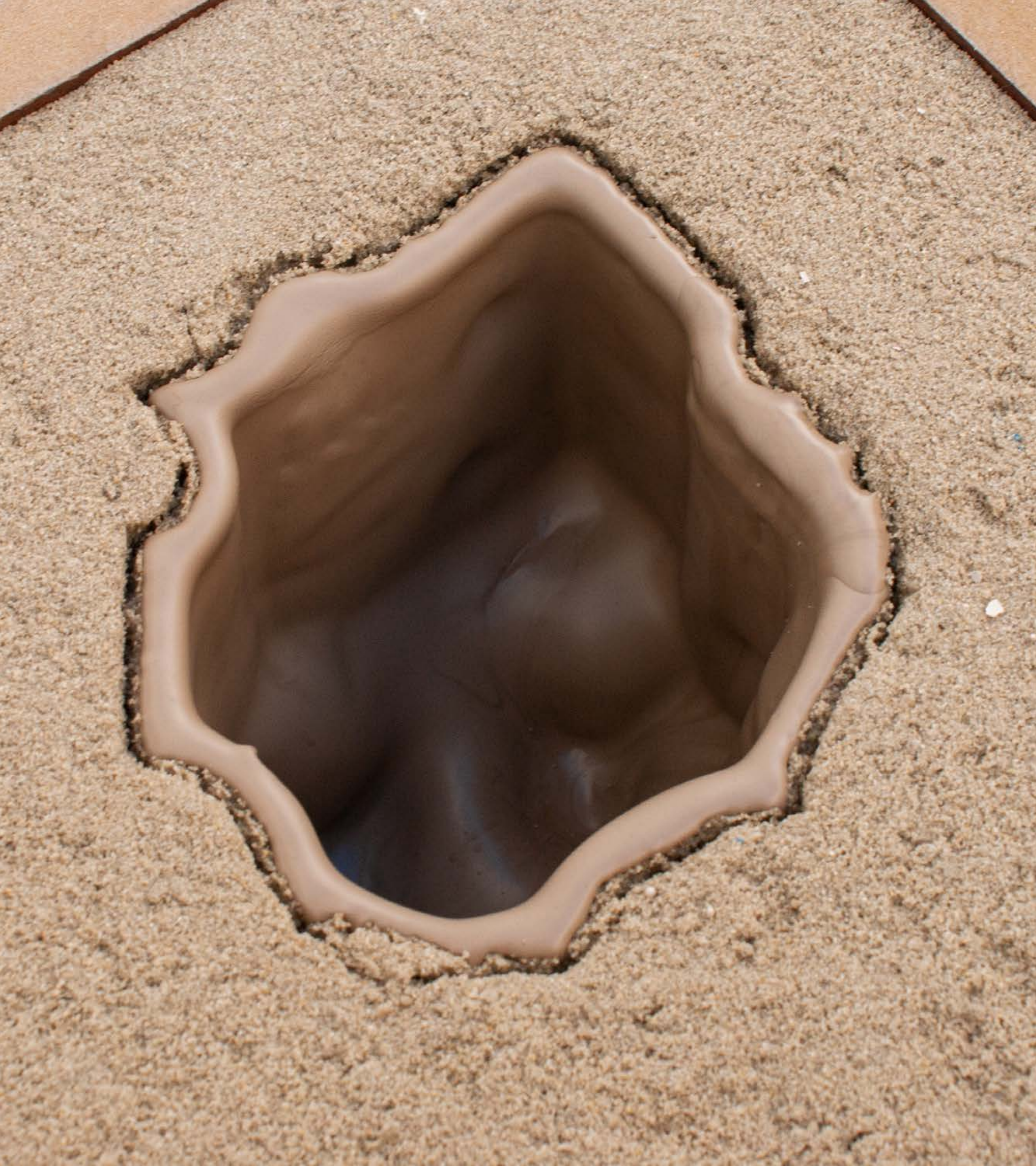
LEFT Cast ready to be “excavated” from sand mould
