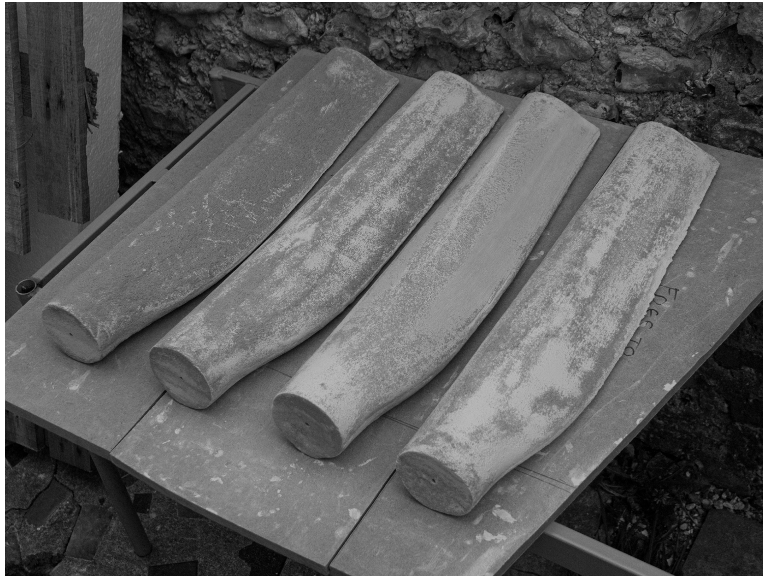
Sand-cast turbine blade sections drying before bisque firing
