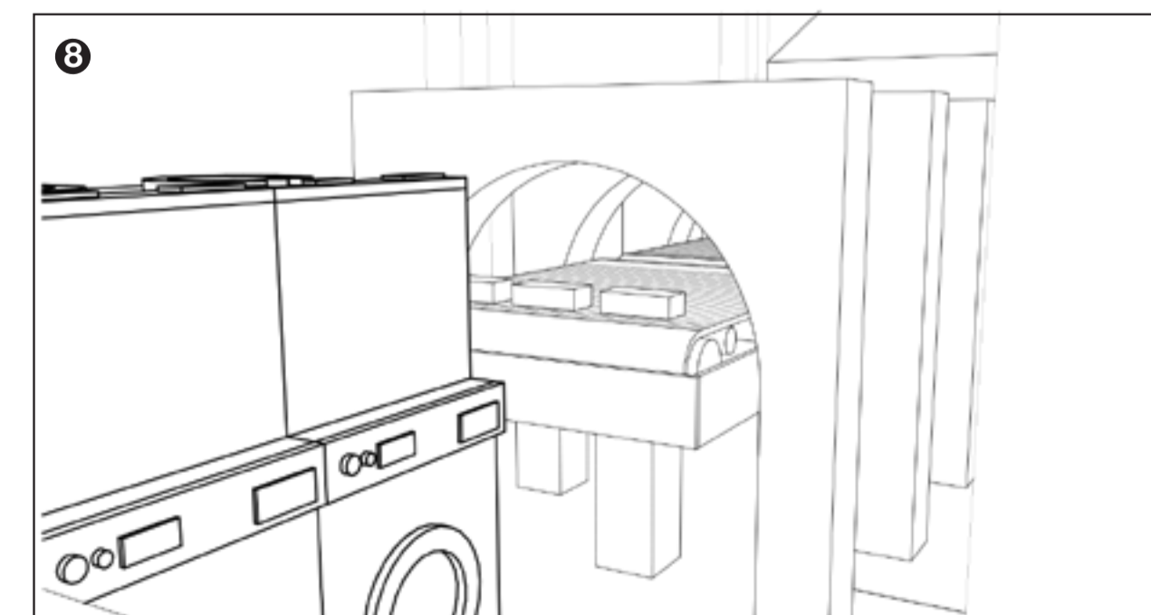
8 When both elements (plastic and excavated material) are broken up into small enough pieces, they get measured out and added to a small amount of cement and water. All the elements get put into the washing machines which act as mixers.
