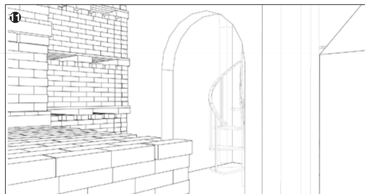
11 The bricks are taken out on the other side of the kiln which is in the storage space. Bricks are left to cool down before being stacked.
